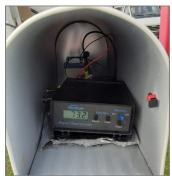
This site on runs off of solar energy that charges a battery and connects to the temperature readout. The solar panel method is more energy efficient and allows for more accurate readings each day. The temperature display is called a NIMBUS and can save up to a month worth of daily observations.
