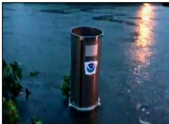
**Figure 3:** Rain gauge in danger of floating away
