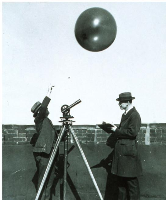
*This image shows early testing of hydrogen-filled balloons for radiosonde measurements. The theodolite in the image was used to track the balloon to the limit of visibility.*
