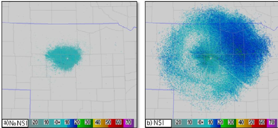
**Figure 1.** WSR-88D 0.5 degree reflectivity image showing (a) standard atmospheric conditions or no NSI and (b) a strong NSI.
