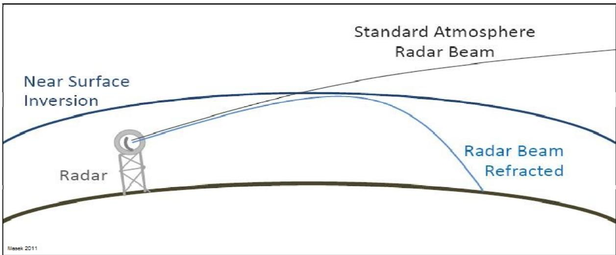
**Figure 2.** Standard atmosphere radar beam and near surface inversion causing super-refracted radar beam.
