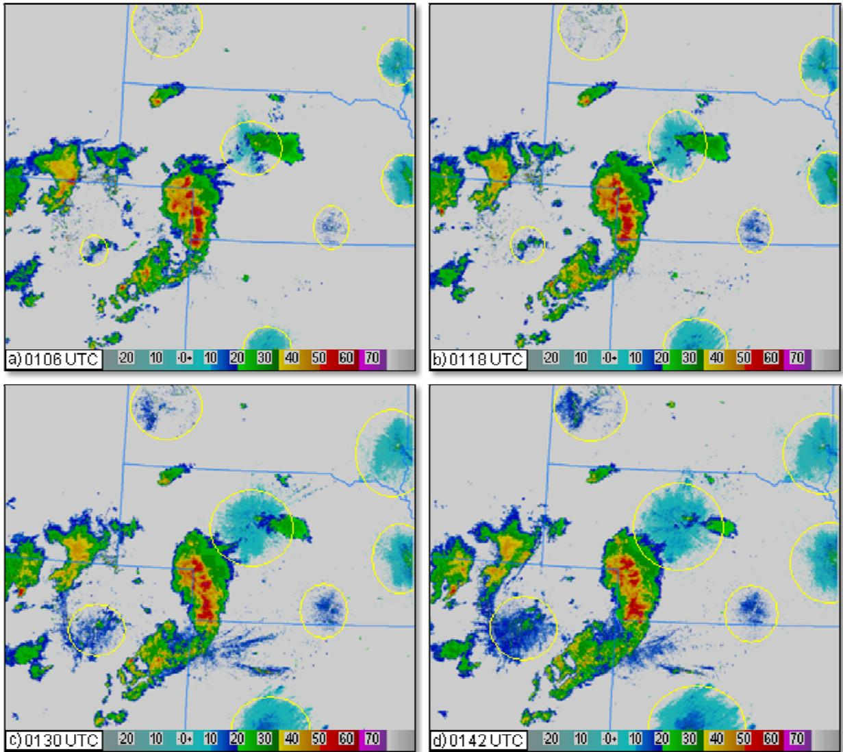
**Figure 9.** 17 September 2007 regional radar for (a) 0106 UTC, (b) 0118 UTC, (c) 0130 UTC and (d) 0142 UTC (AP clutter highlighted in yellow).
