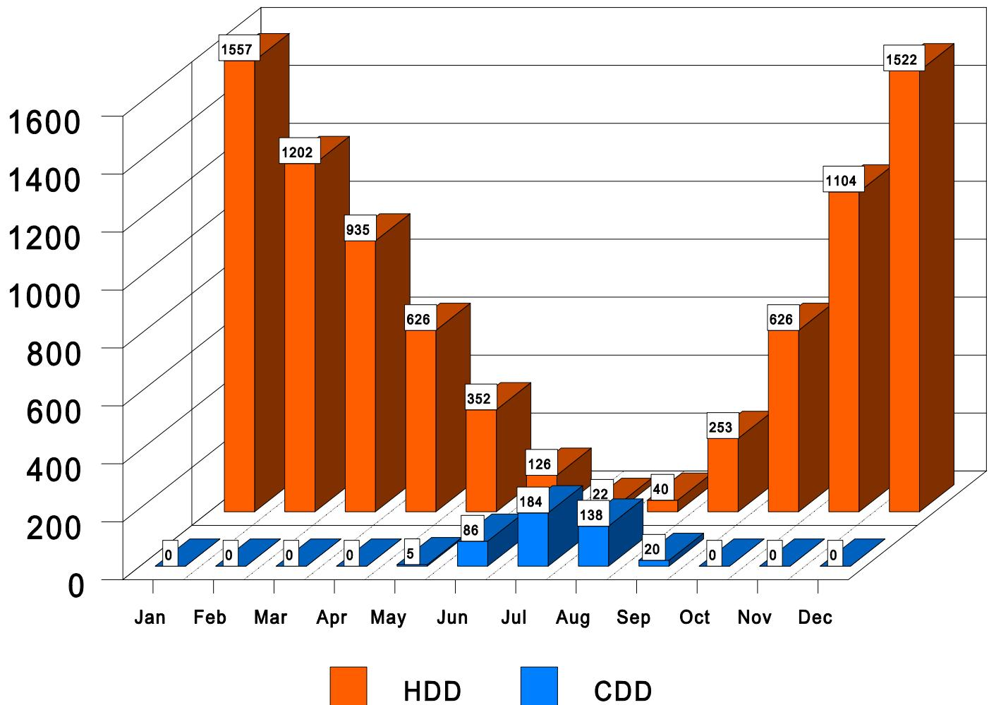
Figure 5. Heating and Cooling Degree Days (based on 65 degree average temperature using 1971-2000 Normals).
