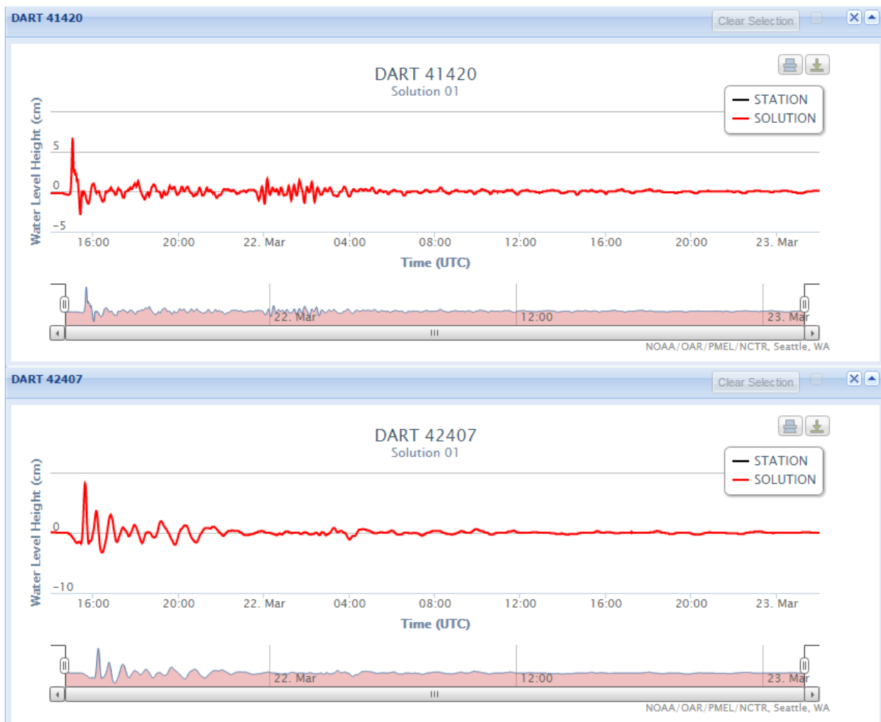
Figure 8. Pairs of time series for DART buoys in the vicinity of Northeastern Lesser Antilles. From top to bottom: DART 41421, 41420, and 42407. The x-axis represents time (UTC) and the y-axis represents the water sea level change in centimeters (cm).
