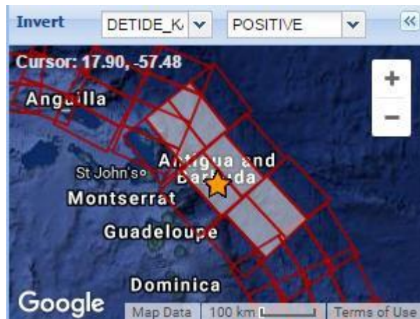
Figure 3. Northeastern Lesser Antilles scenario. Selected unit sources are depicted in frosted rectangles. From top to bottom and left to right: at44a, at43a, at42a, at44z, at43z, and at42z, with boxes measuring 100 km long and 50km wide.
