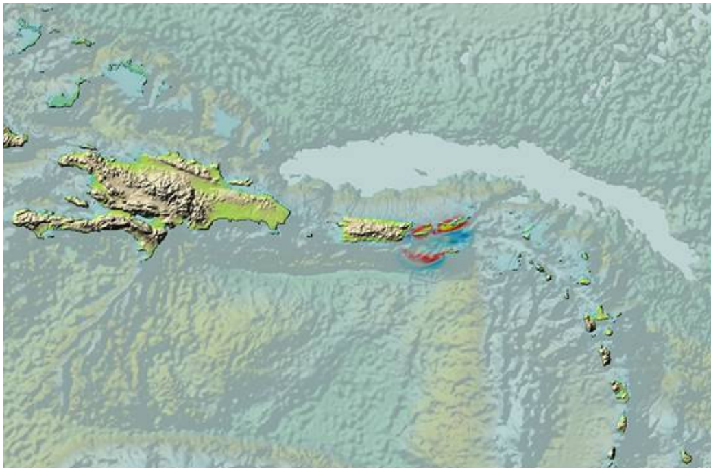
Figure IV-2: Tsunami at ten minutes.
