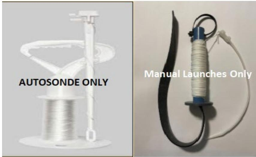
*Figure A-6: Types of Unwinders / Dereelers*
