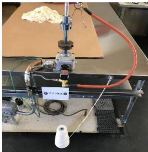
*Figure K- 4 - Typical Fill Valve with approved hose to nozzle, 1/4 turn isolation valve, fill pressure gauge, stainless steel grounded table, and classified fill controller/solenoid*
