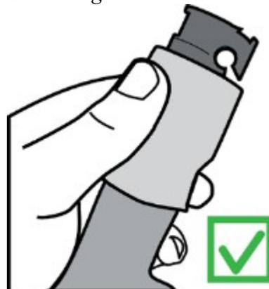
*Figure C-13: Balloon Neck Correctly Folded over the Ring*
