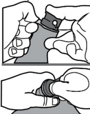
*Figure C-10: Inserting Balloon Nozzle on the Balloon Neck*
