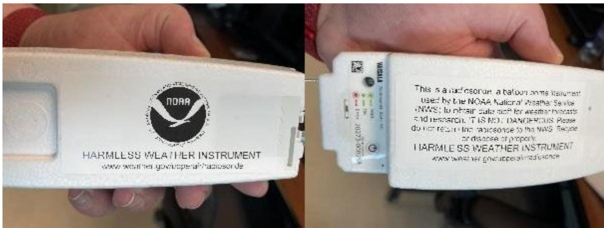
Figure A-2: Upper Air Radiosonde (Vaisala)
