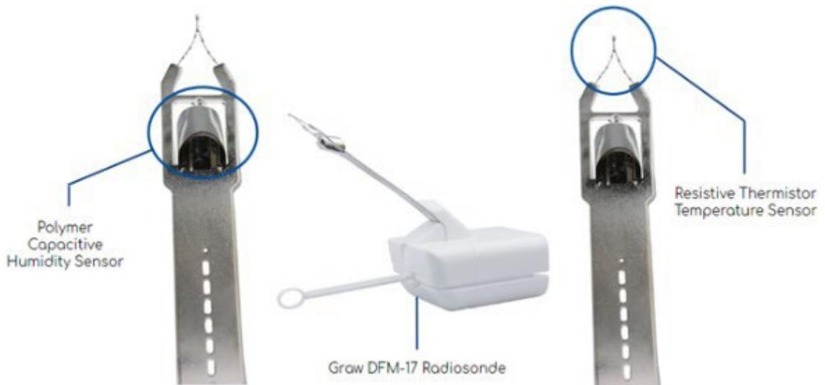
Figure A-4: Radiosonde Sensors (GRAW)
