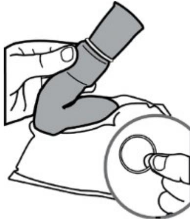
*Figure C-11: Inserting the Nozzle Ring*
