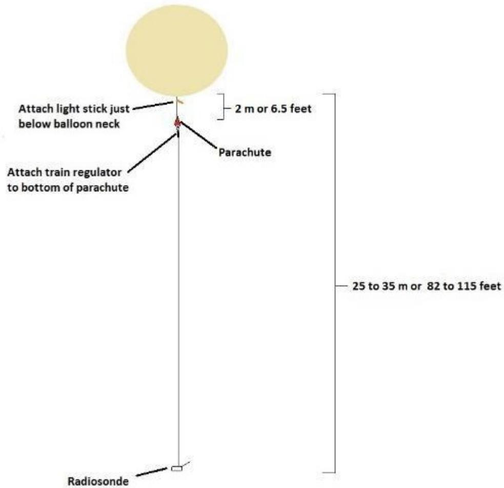
Figure C-3: NWS Flight Train Diagram
