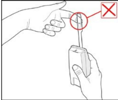
*Figure C-14: Do not Touch the Radiosonde Sensors*
