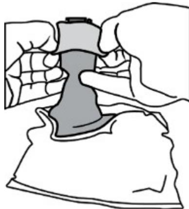
*Figure C-12: Folding the Balloon Neck over the Ring*
