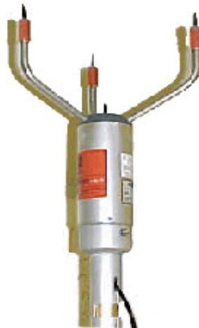
Figure J-3: Vaisala Handar Wind Sensor
