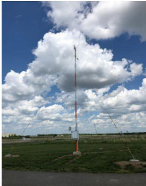
Figure B-6: Vaisala Automatic Weather Station (AWS)
