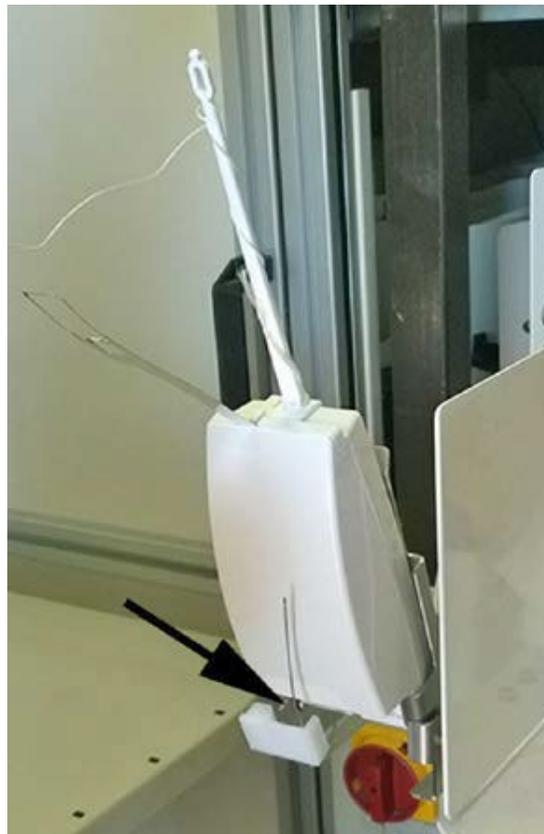
*Figure C-19: Correct Placement of the Radiosonde Antenna*
