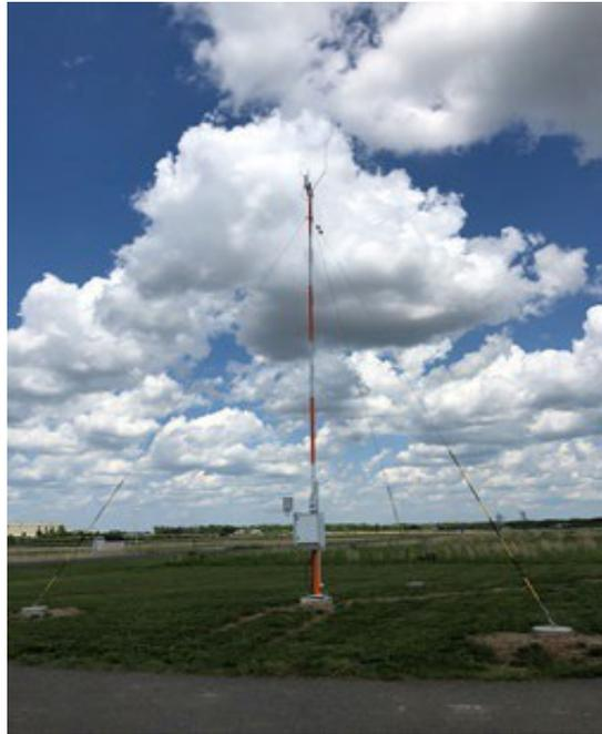
*Figure J-10: Automatic Weather Station (AWS)*
