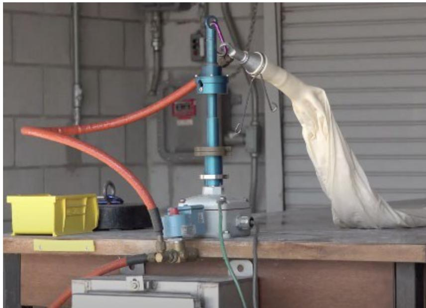
*Figure C-1: Balloon on Inflation Table Secured w/Clamp*
