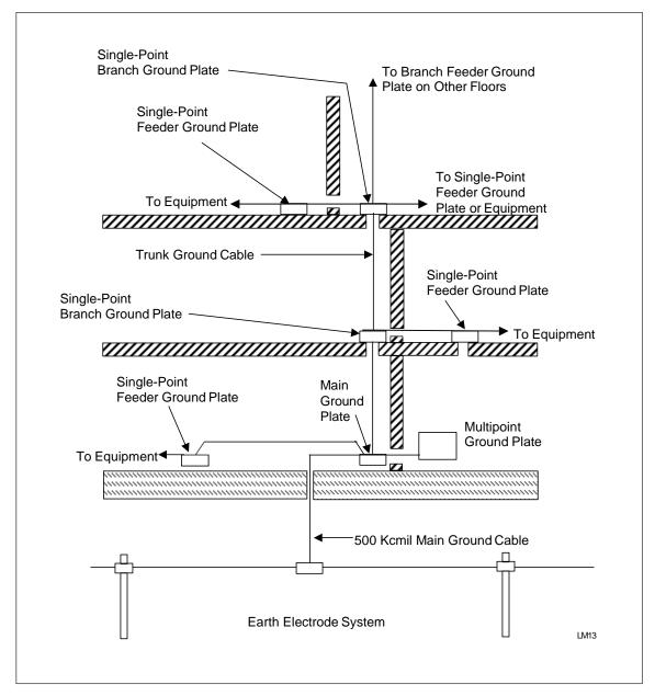
Figure 2-14. Electronic Single-Point Ground System Installation
