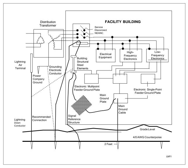
Figure 2-12. Facility Grounding System
