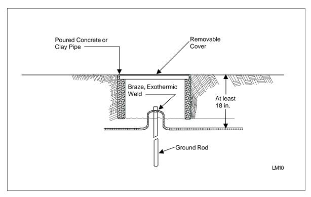
Figure 2-11. Concrete Grounding Access Well
