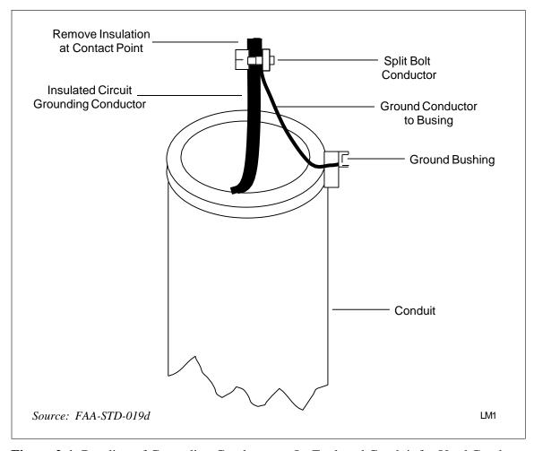
Figure 2-1. Bonding of Grounding Conductor to Its Enclosed Conduit for Used Conductors
