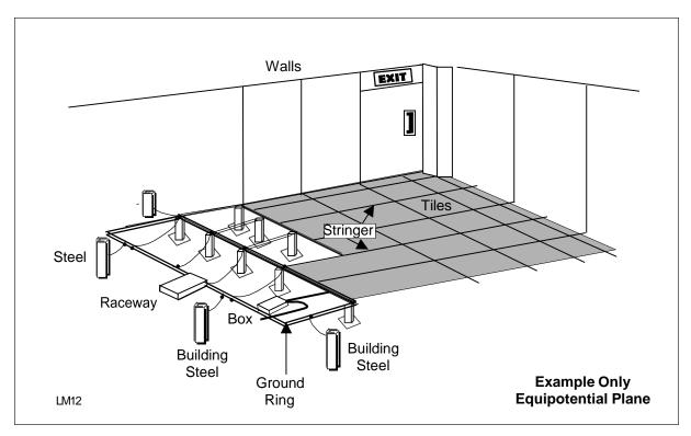
Figure 2-13. Grounding Ring Used for a Signal Reference Grid
