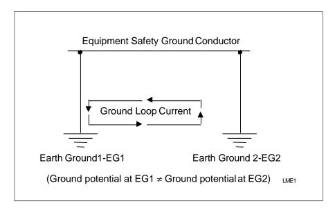
With Earth Ground 1 at a different potential than Earth Ground 2, current flows in the equipment safety ground conductor. This current causes ground noise.
