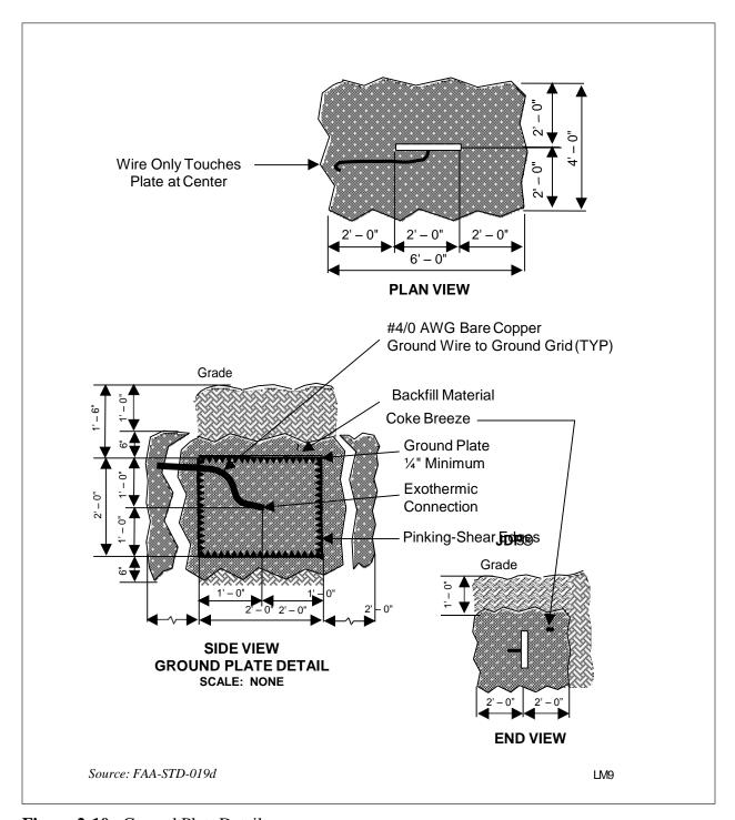
Figure 2-10. Ground Plate Detail
