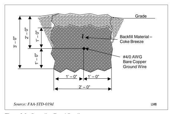
Figure 2-9. Grounding Trench Detail
