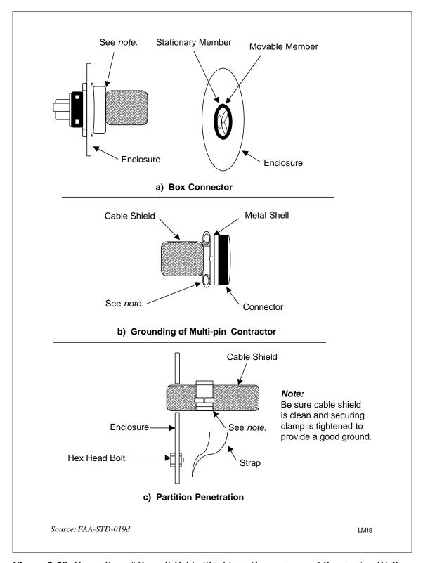
Figure 2-20. Grounding of Overall Cable Shields to Connectors and Penetrating Walls
