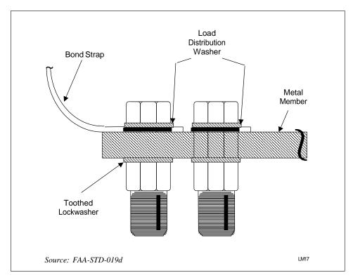
Figure 2-18. Order of Assembly for Bolted Connections
