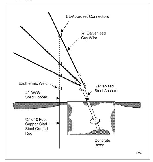
Figure 2-5. Multiple Guy Wire and Anchor Grounding
