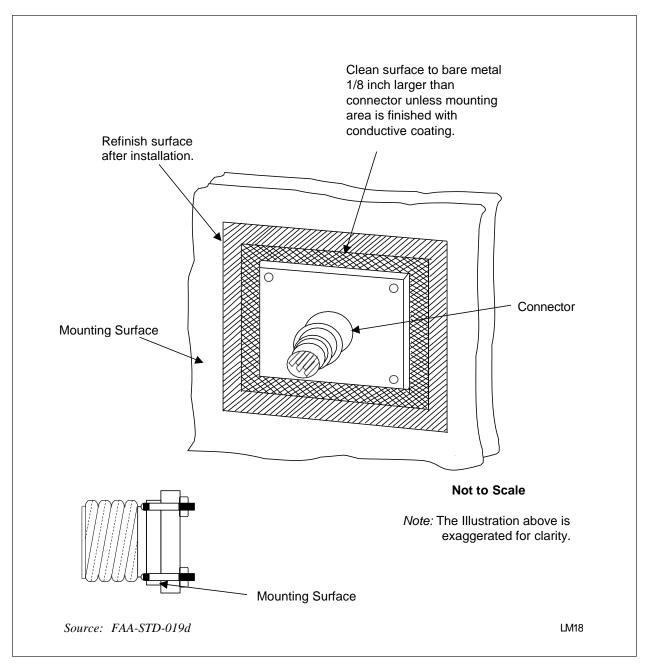
Figure 2-19. Bonding of Connectors to Mounting Surface
