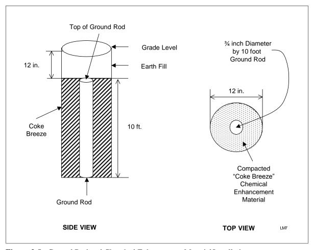
Figure 2-8. Ground Rod and Chemical Enhancement Material Installation
