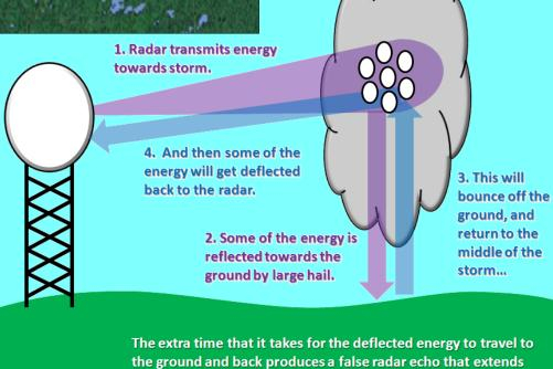
like a spike along a line from the radar to the storm.
