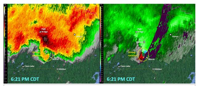
The image on the left is the 0.5 degree reflectivity from the Duluth radar, and the image on the right is the 0.5 storm relative velocity from the Duluth radar. The green velocity data indicates winds that are flowing towards the radar (in this case located off the image to the northwest), and the red velocity data indicates winds that are flowing away from the radar.
