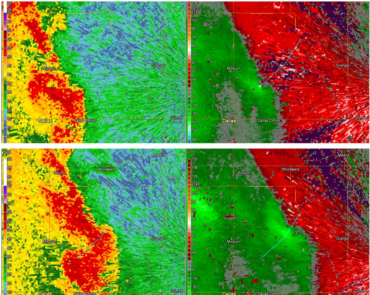
*A sequence of images from the Des Moines WSR-88D radar during the life of the tornado. The path of the tornado is overlaid for comparison. Left image is base reflectivity and the right image is storm-relative velocity. Times are 10:21pm CDT and 10:25pm CDT.*
