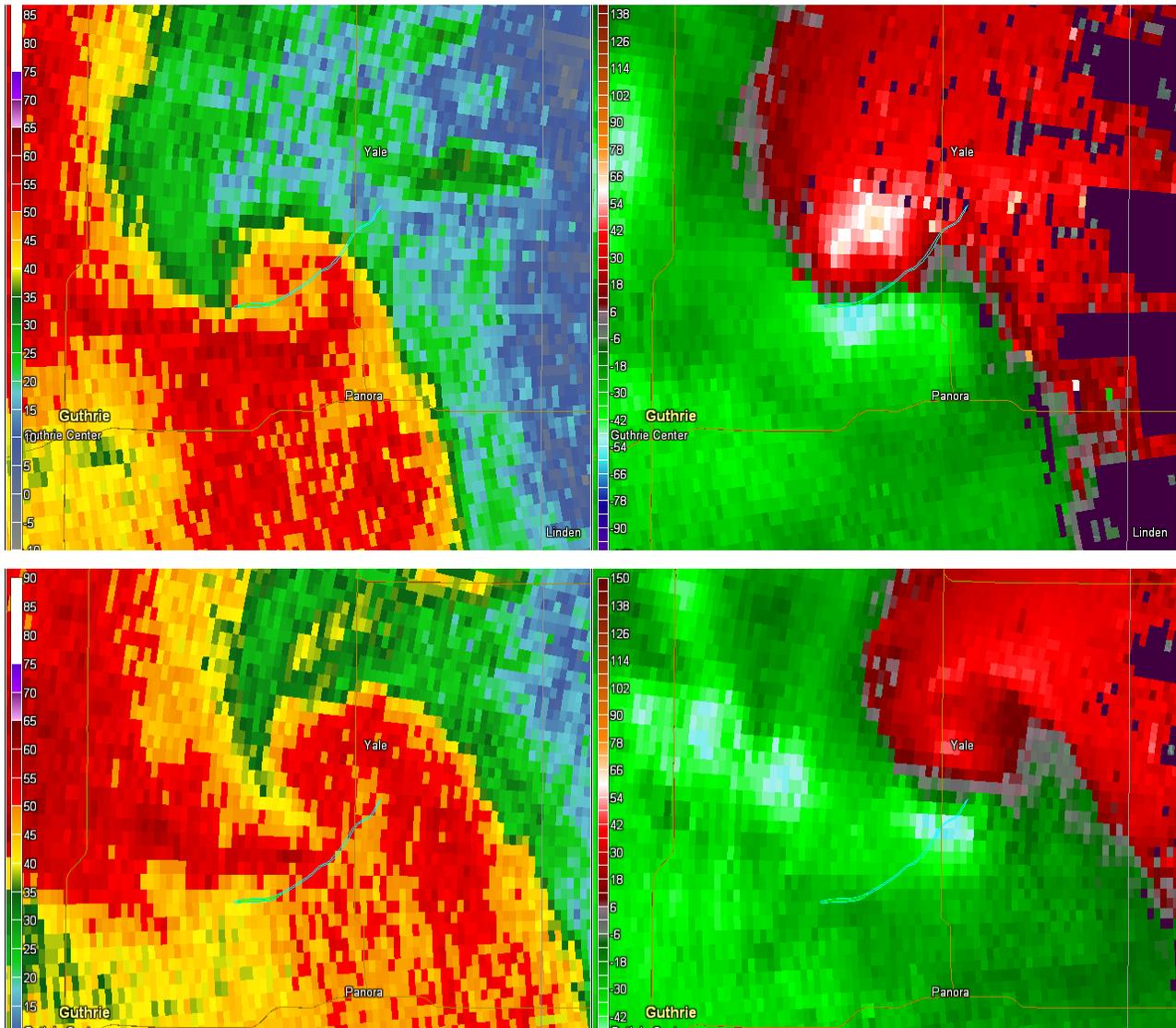
*A sequence of images from the Des Moines WSR-88D radar during the life of the tornado. The path of the tornado is overlaid for comparison. Left image is base reflectivity and the right image is storm-relative velocity. Times are 9:57pm CDT and 10:02pm CDT.*
