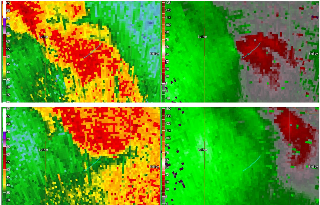
*A sequence of images from the Des Moines WSR-88D radar during the life of the tornado. The path of the tornado is overlaid for comparison. Left image is base reflectivity and the right image is storm-relative velocity. Times are 10:44pm CDT and 10:49pm CDT.*
