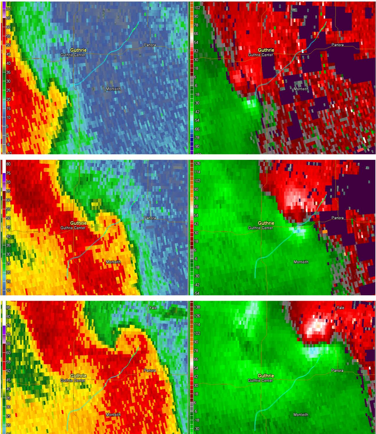
*A sequence of images from the Des Moines WSR-88D radar during the life of the tornado. The path of the tornado is overlaid for comparison. Left image is base reflectivity and the right image is storm-relative velocity. Times are 9:43pm CDT, 9:53pm CDT, and 9:57pm CDT.*
