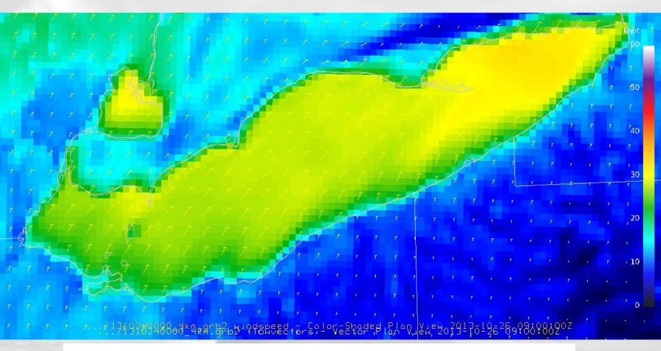
Boundary layer growth not as abrupt as the 12km representation - signifying smaller scale processes are really at play in the growth of the mixing layer.
