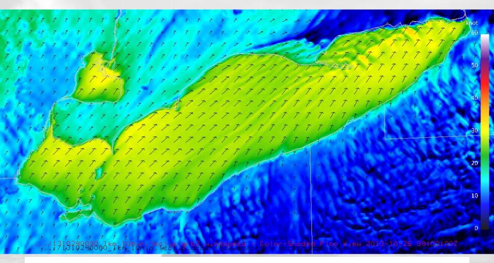
Refined detail indicating formation of convective roll structures are responsible for the momentum transport to the surface rather than slab overturning as shown in the coarse domain.
