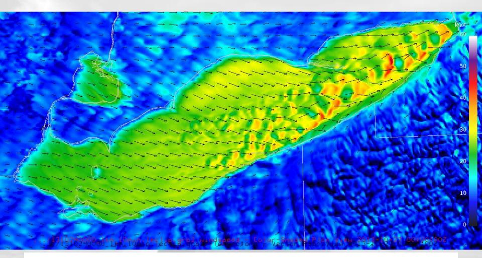
Refined detail indicating formation of cellular convection is responsible for the momentum transport to the surface rather than slab overturning as shown in the coarse domain.
