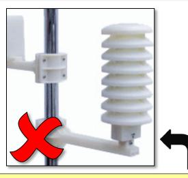
While the sensor above *is* in a radiation shield, it is too small, with little space for proper airflow. It will likely report erroneously warm temperatures during the day.
