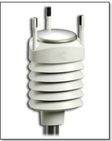
Sonic Anemometers (left) are still fairly rare (and expensive), but are less likely to fail from icing. However, birds perching on the sensor probes can cause problems, and extremely high false wind gusts!
