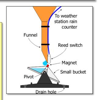
However, there is a drawback to simplicity. In cases of torrential rainfall, some rain may be lost "between tips." This will result in a low-bias in ALL tipping bucket rain gauges. It is always good to have a standard rain gauge for final precipitation amounts... but standard rain gauges can't report live data!
