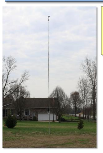
**LEFT:** This sensor suite is far from obstructions, with the anemometer mounted at about 10 m, and temp/humidity/rain gauge sensor suite about 5-6 feet AGL. Hopefully there are cable stays to prevent wobbling.
