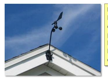
**LEFT:** This anemometer is mounted far too low relative to the roof line. The wind direction will be heavily influenced by the peak of the roof, and the wind speed will be erratic as the roof may enhance or block the wind, depending on the direction.
