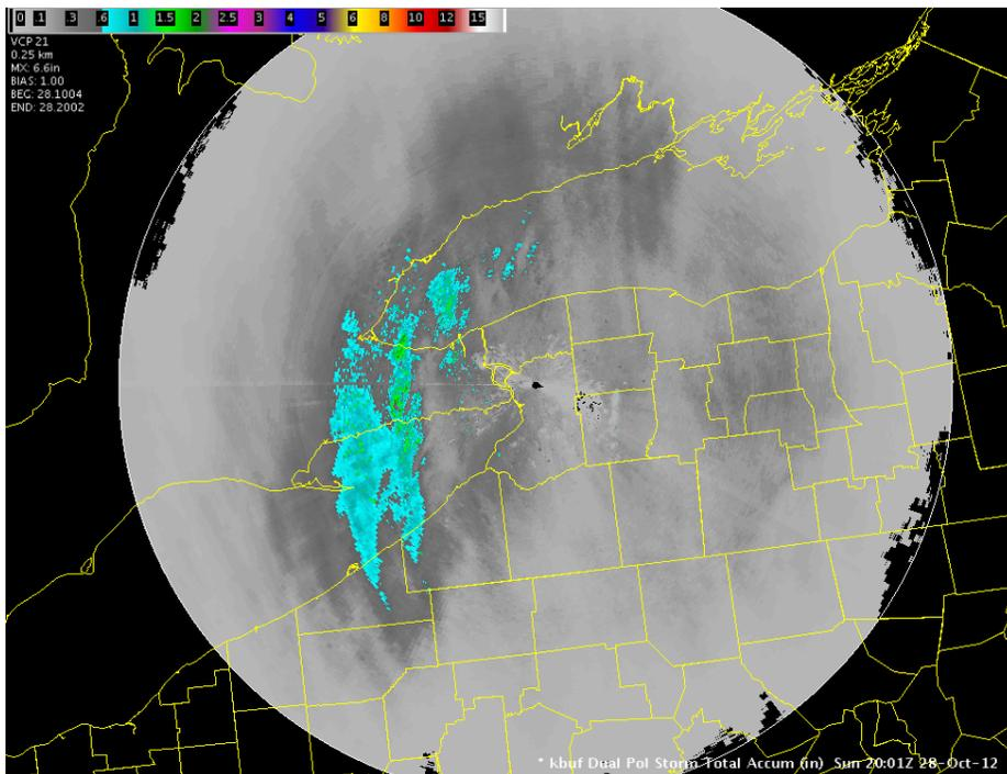
**Figure 5.** DP Storm Total Precipitation QPE from the Buffalo radar on October 28<sup>th</sup>, 2012 between 1004Z and 2002Z. This is the same event but using a multiplier of 1.5 for snow and ice crystals. Note the reduction of the melting layer discontinuity ring.
