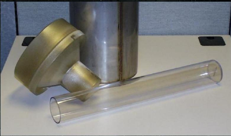
First, let's see how many of you have a keen eye and recognize that gage #4 isn't a rain gage at all, rather a "bee-hive" enclosure for a thermistor that measures temperature! These devices are used for our nationwide Cooperative Observer program and are part of what's called an MMTS or Maximum Minimum Temperature System.
