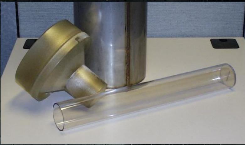
First, let's see how many of you have a keen eye and recognize that gage #4 isn't a rain gage at all, rather a "bee-hive" enclosure for a thermistor that measures temperature! These devices are used for our nationwide Cooperative Observer program and are part of what's called an MMTS or Maximum Minimum Temperature System.
