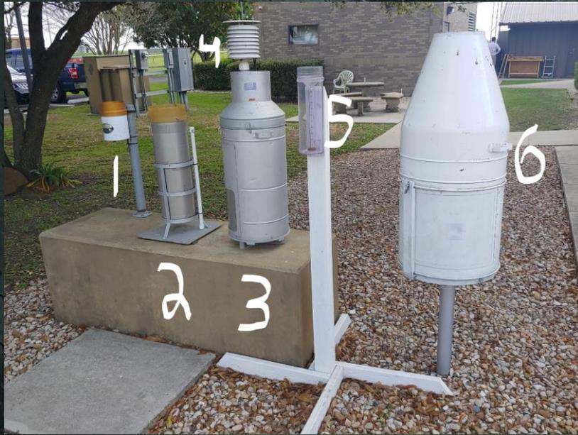
Gage #1 is a "Tipping Bucket" gage, and it's our most commonly used *near-real time automated* rainfall measurement device. The gold top portion is a funnel that drips down into a little triangular "bucket" that tips over and empties once it's reached a set amount. After tipping, a second "bucket" faces up, which repeats the process and tips back when full (see the schematic below.)
