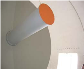
RRS parabolic dish with narrow angle gathering feed horn.
