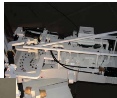
(Left and above) New components added to the NWS Doppler radar to give it dual-polarization capabilities.
