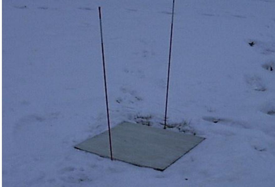
An example of a snowboard and how to mark where it is.
