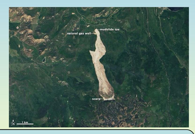
On May 25, 2014, a large landslide occurred near the town of Collbran covering an area three miles long and three-quarter of a mile wide. It claimed the lives of three people. Rainfall estimates near the slide were ~ 1 inch (2.5 cm). However, antecedent moisture, moist ground due to runoff, and unstable geology were believed to be the main factors which caused the slide.
