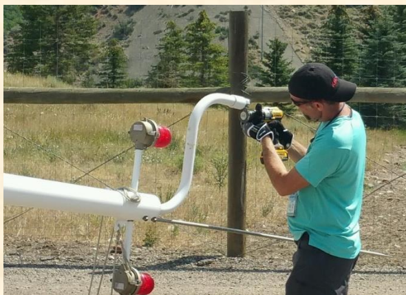
Image 1: ET Mike Martinez using a cordless drill to sand the edges of the alignment collar of an ASOS so the new IFWS will fit properly. Photo credit: NWS.
