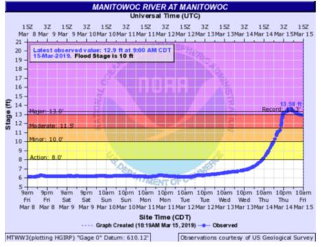
Figure 2: Hydrograph depicting the record crest on the Manitowoc River at Manitowoc.
