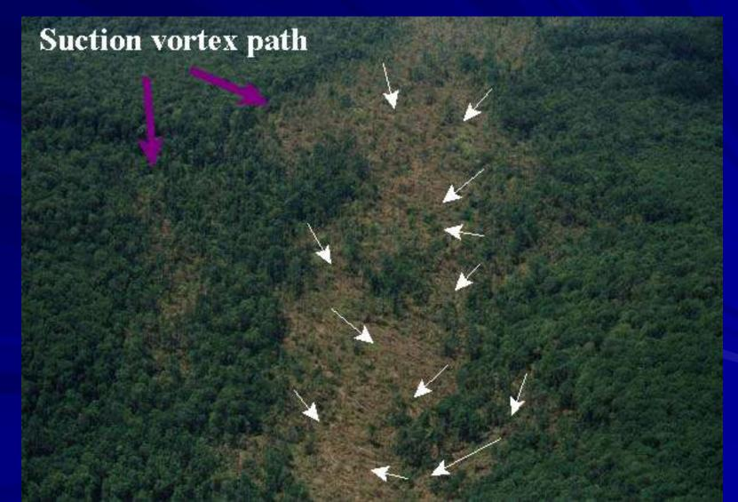
The fan-shaped, divergent tree fall pattern that is typical of a microburst, as seen from the air:
