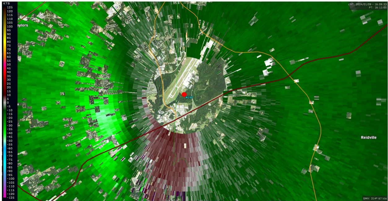
Fig. 29. Base velocity (kts; 0.2° scan) from KGSP (red dot) at 1611 UTC with 50 kts at 56 ft ARL approaching the radar.
