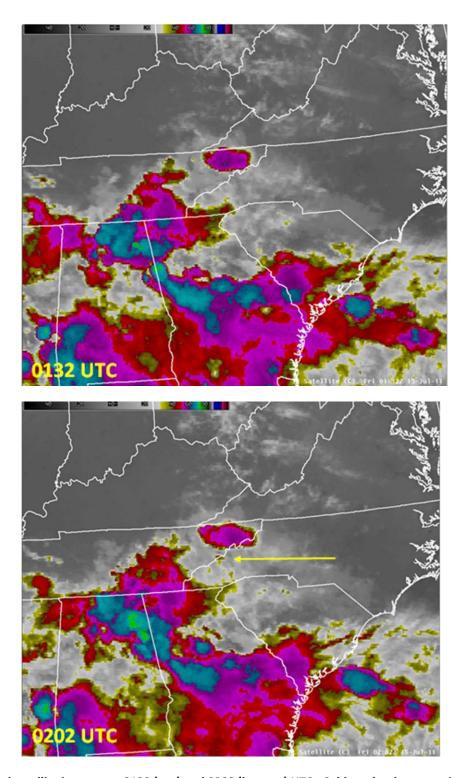
Fig. 16. Infrared satellite imagery at 0132 (top) and 0202 (bottom) UTC. Coldest cloud tops are in purple and blue shades. Arrow in bottom panel points toward expanding cold cloud top (-46°C) in the vicinity of Straight Fork Creek headwaters. The GOES-East viewing angle results in cloud features being offset slightly northward from their actual position relative to the earth.
