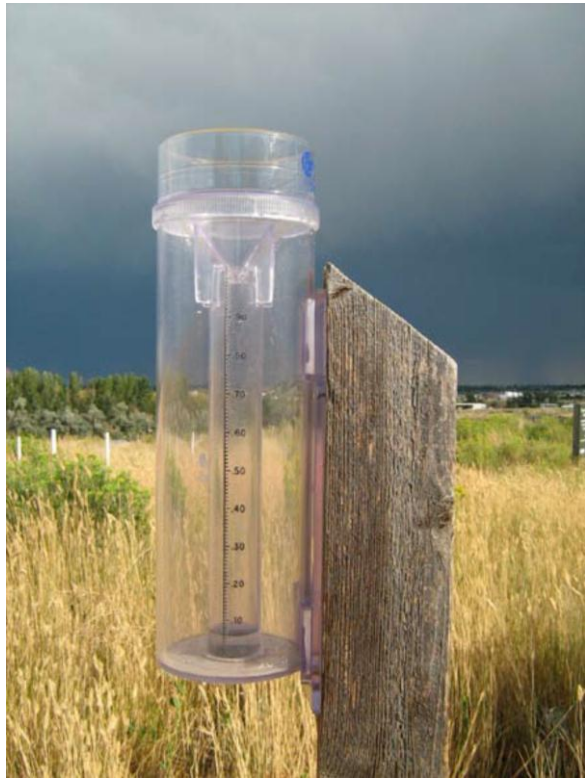
Figure 3: A well placed rain gage is far from any obstructions (including trees and fences), 4 to 5 feet off the ground, and level.
