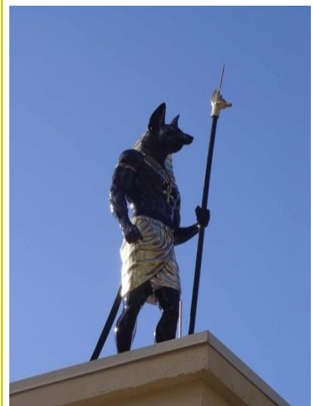
Figure 7: Statues and spires at Storyland are not just there for decoration. They are also there to serve as lightning rods to protect patrons from lightning.
