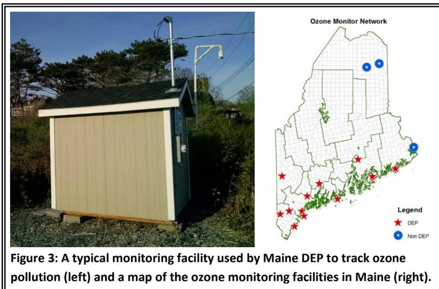
**Figure 3: A typical monitoring facility used by Maine DEP to track ozone pollution (left) and a map of the ozone monitoring facilities in Maine (right).**
