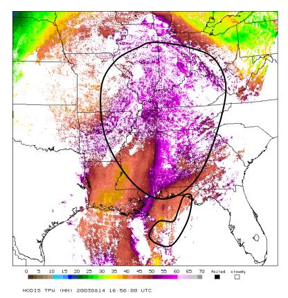
Figure 4. Total precipitable water (mm) derived from GOES (top) at 1546UTC and Terra MODIS (bottom) at 1656UTC on August 14, 2003. The GOES product is at 10km and the MODIS at 1km resolution. The highlighted box on the GOES product indicates the region of MODIS coverage.
