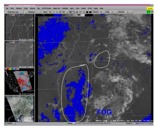
Figure 2. MODIS 11-3.9 $\mu$ m difference image at 0728UTC on August 14, 2003 displayed in AWIPS. The enhanced blue portions of the image indicate regions of ground fog. These regions correspond well with surface observations of reduced visibility (not shown).
