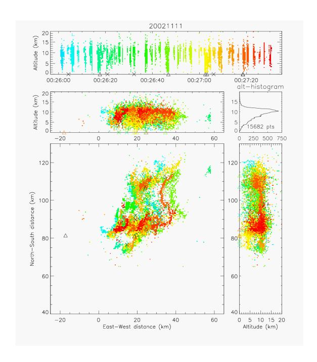
**Fig. 4.** Locations of LMA VHF sources in cell E within a 90 s interval (0026:00-0027:30 UTC). Vertical projections above and right of base map shows VHF source density as a function of E-W and N-S distance versus altitude (km). NLDN ground strike polarity is also shown (triangle for negative CG, X for positive CG). A lightning hole is centered at x=13, y=80, near the main updraft of the cell.
