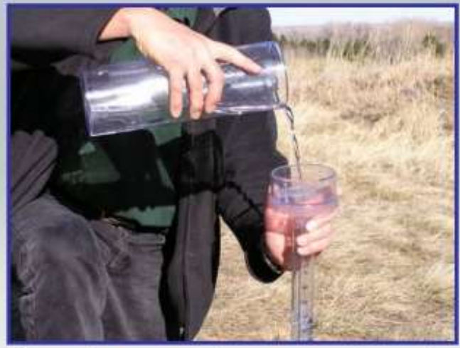
Pour the remaining water into the funnel and measure the inner tube.
