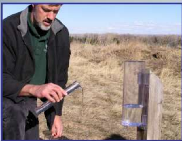
Pour out the first inch from the inner tube and write it down.
