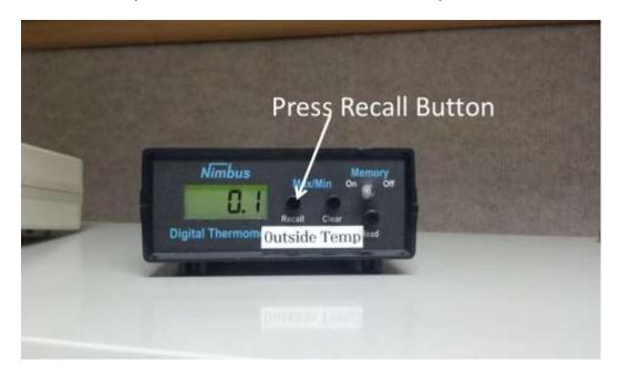
The temperatures displayed prior to 0.1 are the high and low recorded so far from 7am this morning until the current time. This is considered 0 days back or 0.0. We need to go back by one day in order to display the high and low from 7am yesterday morning through 7am this morning. The 0.1 on the display means that the high and low displayed following the 0.1 are the temperatures from one day back or yesterday until today.
