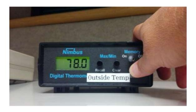
Repeatedly press or hold down the Read button until you see 00:00. Remember we have set the time on the display to read 00:00 when the actual time is 7am. Once you see 00:00, the temperature displayed afterwards was our temperature at 7am this morning. This is your at observation temperature for today's observation. In the below example the temperature at 7am this morning was 68 degrees.
