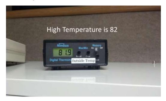
The next press of the Recall button will now display the time the high was recorded. The time is offset and may not make sense since we have the time offset in order for midnight to occur at 7am. We do not need the time for our observation so press the Recall button again to display the low.
