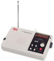
Special radios can be programmed to receive certain alerts for select areas using the Specific Area Message Encoder (SAME) feature, can run on battery (in case of a power failure) and can also be
