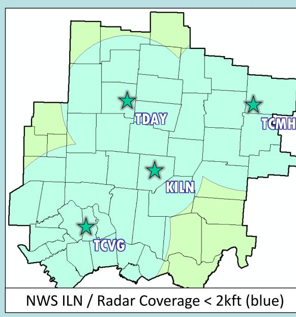
Forty-five TDWRs are installed across the US, with three well-spaced TDWRs within the NWS Wilmington Ohio (ILN) forecast area. Along with the WSR-88D, 80% of the ILN forecast area is covered by radar within 2000 feet of ground level. This makes the ILN forecast area an excellent location for detecting and studying shallow QLCS tornadoes.
