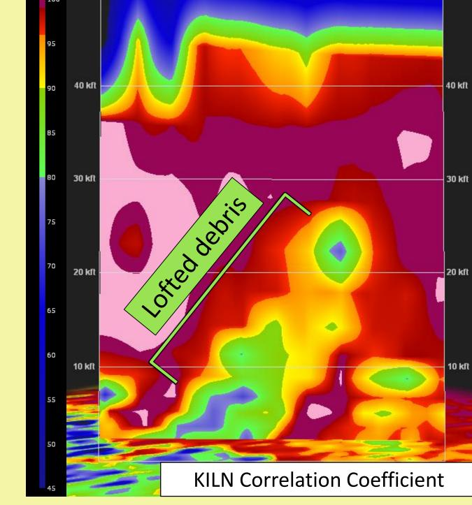
Cross-section radar imagery of the tornado near Trotwood, Ohio at 10:57 PM on May 27, 2019. Reductions of correlation coefficient were observed above 20,000 feet, suggesting a violent (EF4+) tornado.
