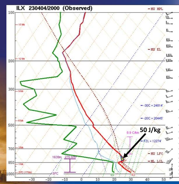
On the flip side...if the brown dashed line is to the left of the red line, that means the parcel is cooler than the environment (stable)
