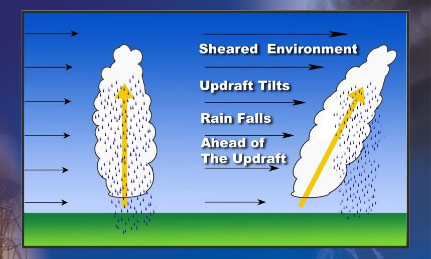
Wind shear acts to tilt thunderstorm updrafts. This prevents rain from falling directly into the updraft...helping it last longer and potentially become stronger
