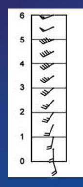
Describes how the wind changes speed and/or direction with height
