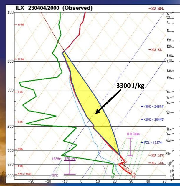
Warm air is less dense (lighter) than cold air. So...if a parcel of air rising from the surface remains warmer than the environment, it will keep rising on its own (hot air balloon)
