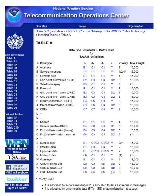
By using the  $T_1T_2A_1A_2ii$  portion of the WMO message, a customer can decode the type of message and the area covered by using the appropriate tables.
