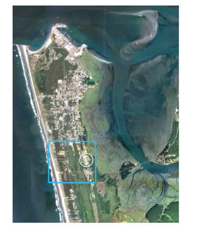
Westport, WA, Google Earth image. Blue rectangle is area of fine resolution GeoClaw tsunami model grid; white circle encompasses Ocosta School campus. Study funded by Washington State Emergency Management Division The next step was to do high-resolution tsunami inundation modeling to define the required height of the structure and to estimate the loads the structure would be designed to resist.
