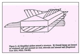
differences are created causing outward pressures forces that can act to lift the roof.
