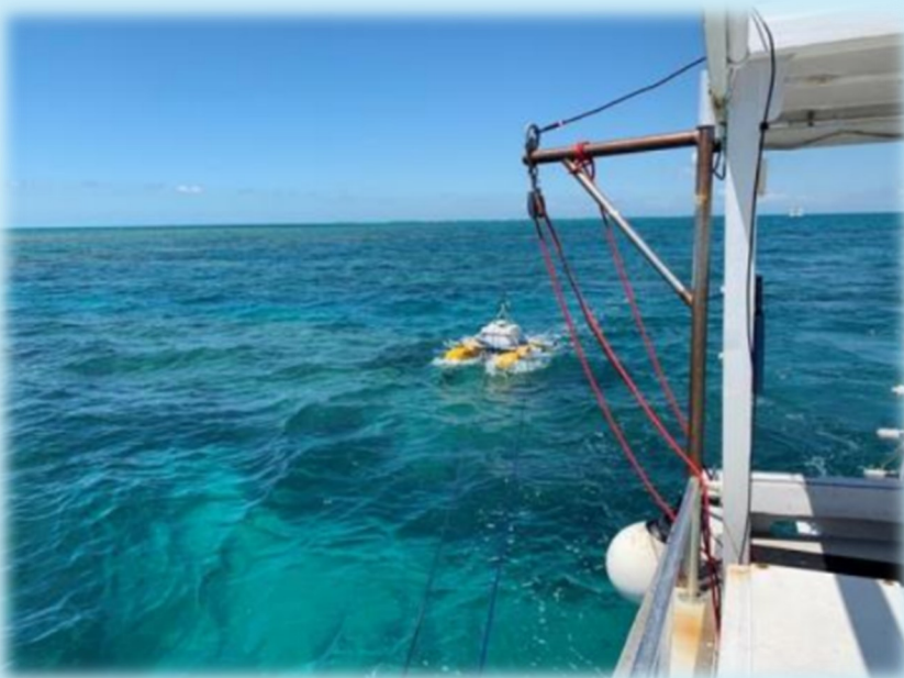
The United States Geological Survey (USGS) SQUID-5 camera system conducting a mission in the Looe Key Sanctuary Preservation Area.
