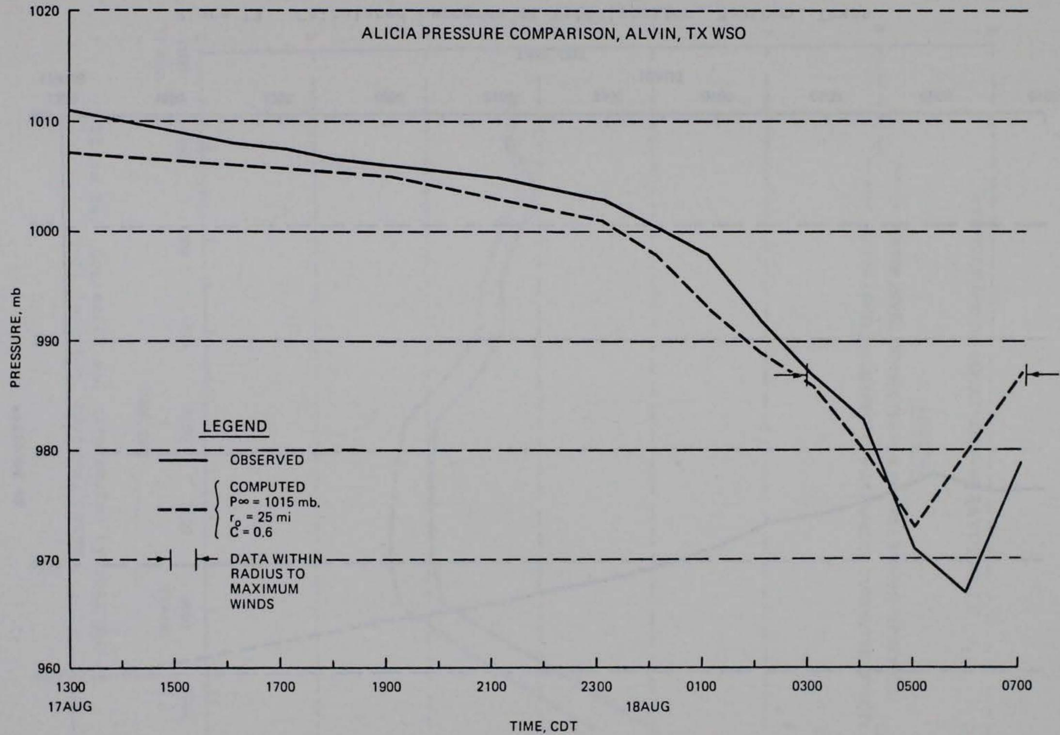
Plate 12. Comparison of observed and computed pressures for Alvin Weather Service Office location
