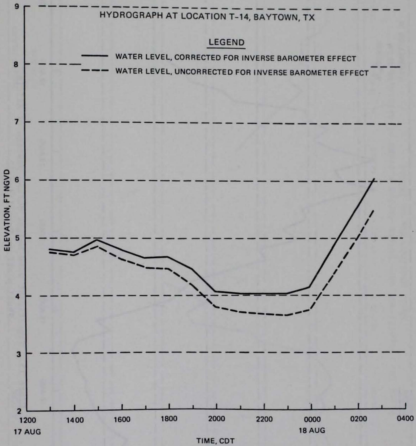
Plate 14. Corrected and uncorrected hydrographs,
