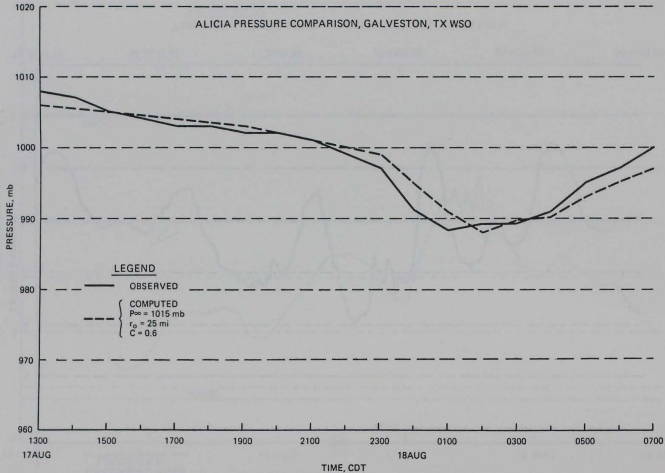
Plate 11. Comparison of observed and computed pressures for Galveston Weather Service Office location
