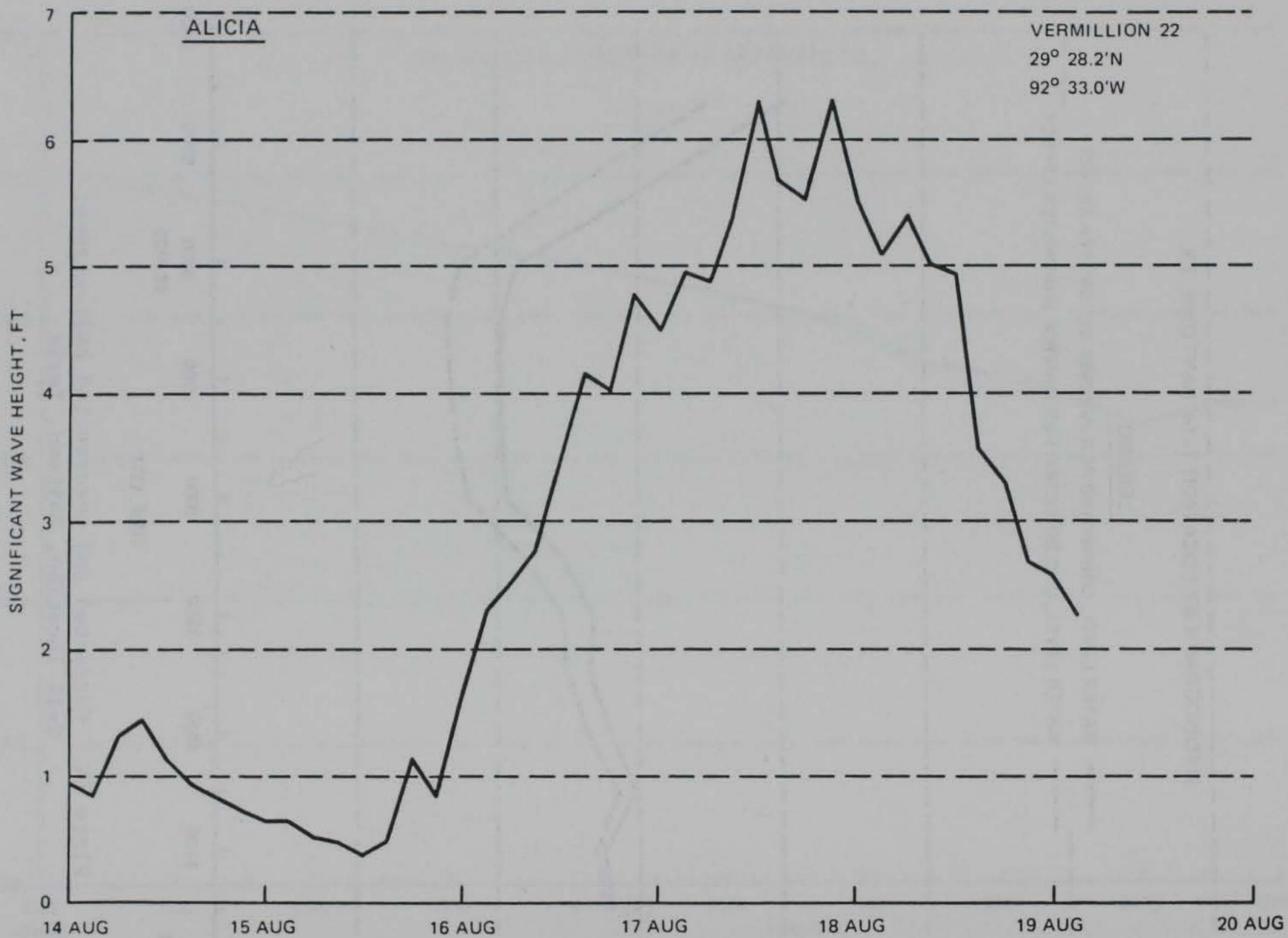
Plate 15. Significant wave height during passage of Alicia,
