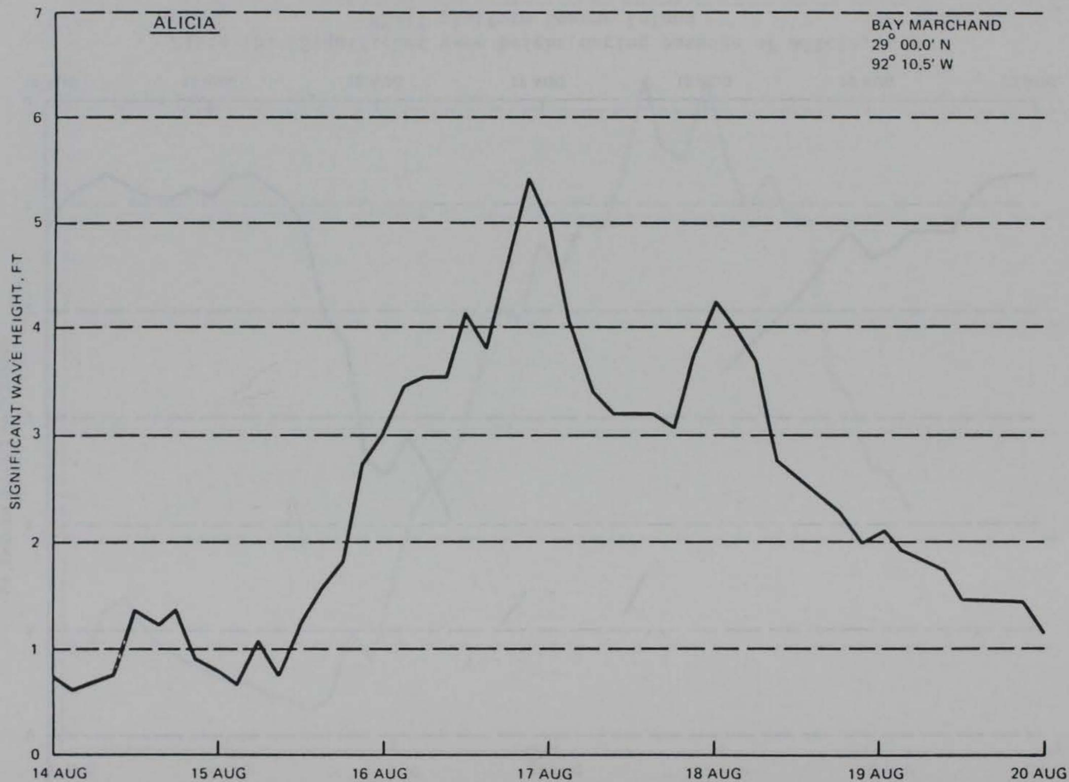
Plate 17. Significant wave height during passage of Alicia,
