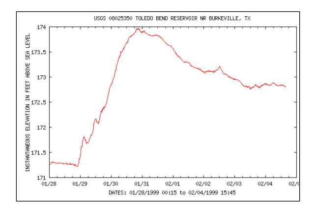
To relieve pressure from the Toledo Bend dam, the spillway gates were opened to release water from the reservoir. This would have an immediate impact on river levels downstream of the dam.
