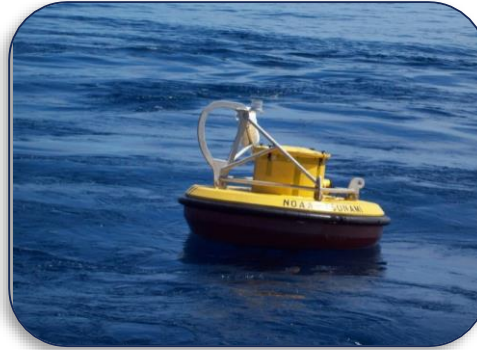
DART buoy and Bottom Pressure Recorder
