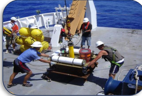
DART buoy and Bottom Pressure Recorder
