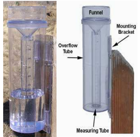
The rain gauge used by CoCoRaHS observers is a simple plastic tube that is easily mounted
