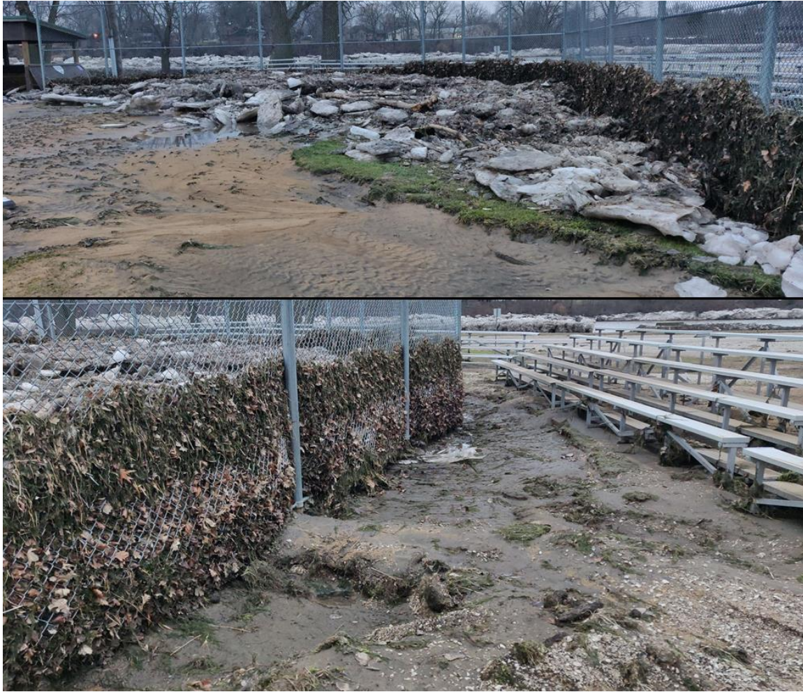
Figure 20. Vegetation stuck in the fence at baseball field at North Island Park (downstream end) in Wilmington. These high water marks suggest a peak water level of about 536 feet elevation. Photographed on January 30.
