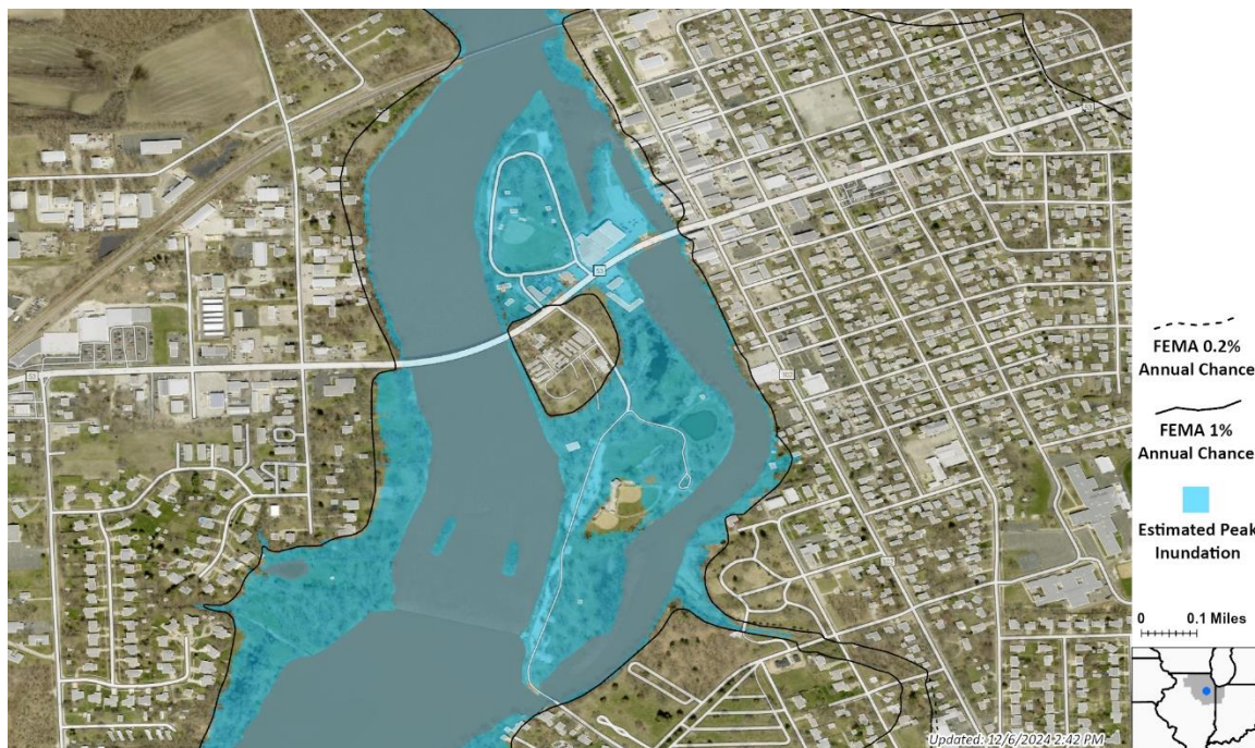
Figure 12. Estimated peak inundation along the lower Kankakee River at Wilmington from the ice jam related flooding of mid-January, 2024. The estimated flood extents associated with the 0.2% annual chance and 1% annual chance floods, as published by FEMA, are added as an overlay.
