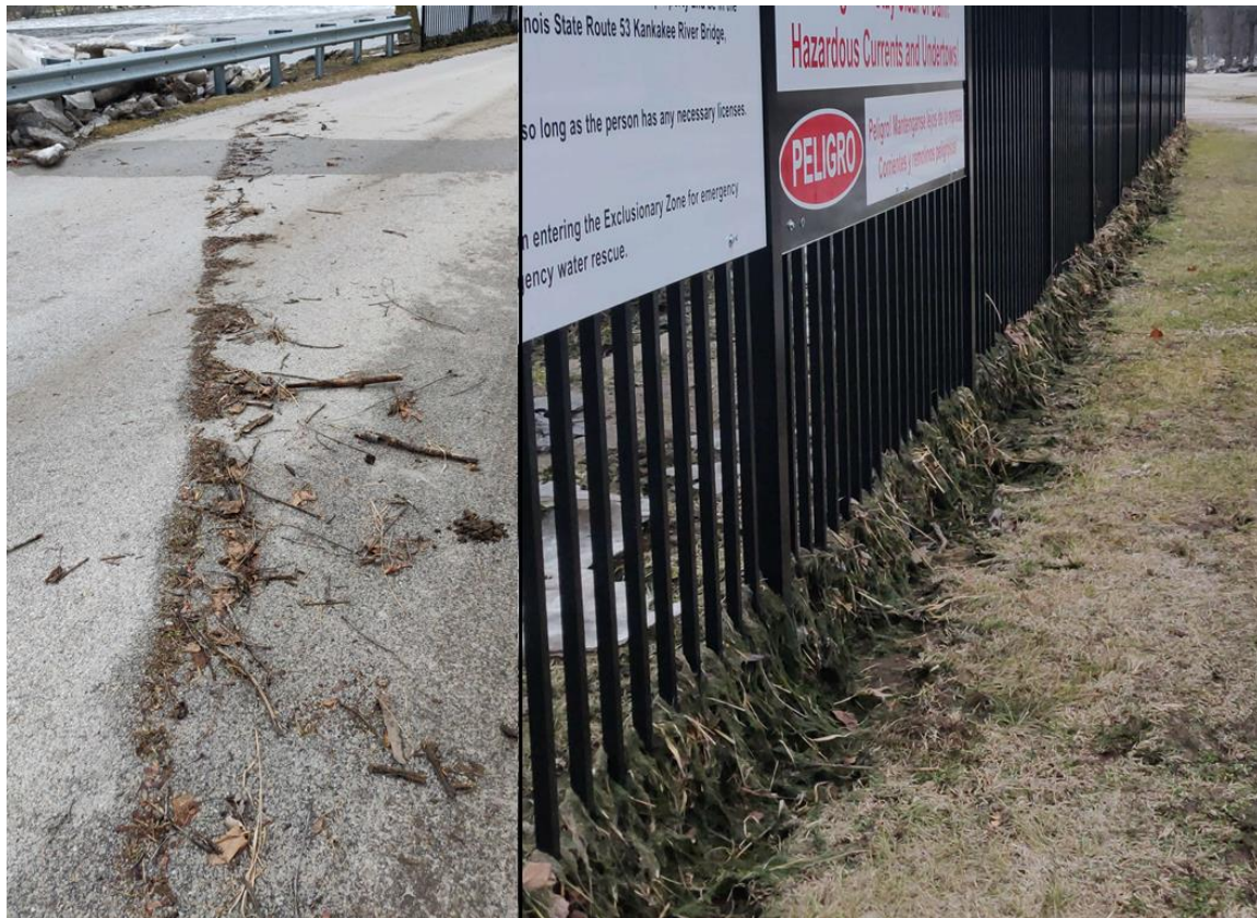
Figure 16. Vegetation debris lines on the roadway in Island Park and vegetation stuck in the fence near Wilmington Dam visible on January 30. These high water marks suggest a peak water level of about 539 feet elevation.
