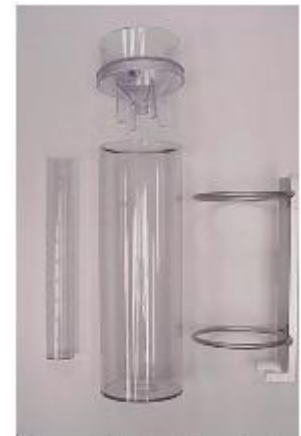
Figure A-7. Four-Inch Plastic Gauge
