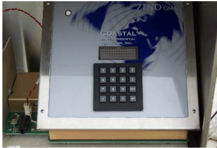
Figure A-18. Data Logger
