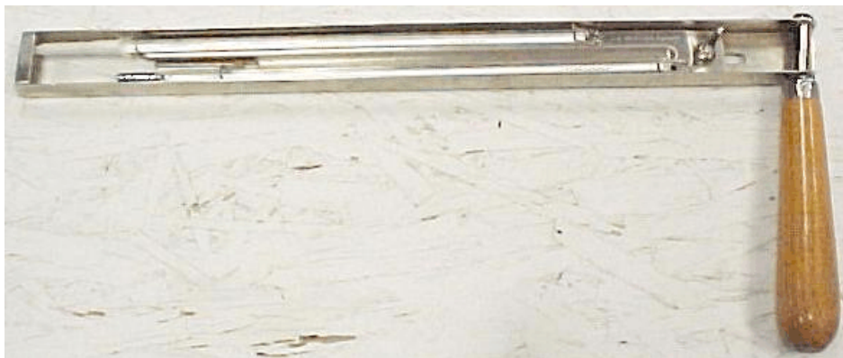
Figure D-10. Sling Psychrometer
