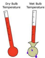
Have you ever seen a thermometer with a sock on the end? The sock is dipped in water, and the mercury drops depending on how much evaporation/cooling occurs. If it's a dry day, there will be lots of evaporation, and not so much when it's humid. The temperature that's measured is the "wet bulb" reading.
