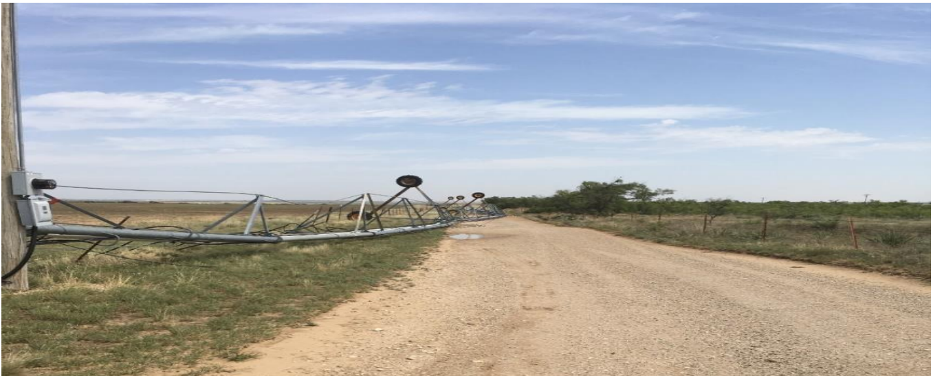
Figure 6. Pivot irrigation system blown onto county road.
