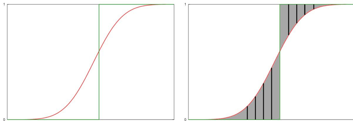
**Fig. 8. An illustration of the computation of Continuous Rank Probability Score for a single forecast case. The red curve is the forecast CDF. The green line is a unit step function located at the value of the verifying observation.**
