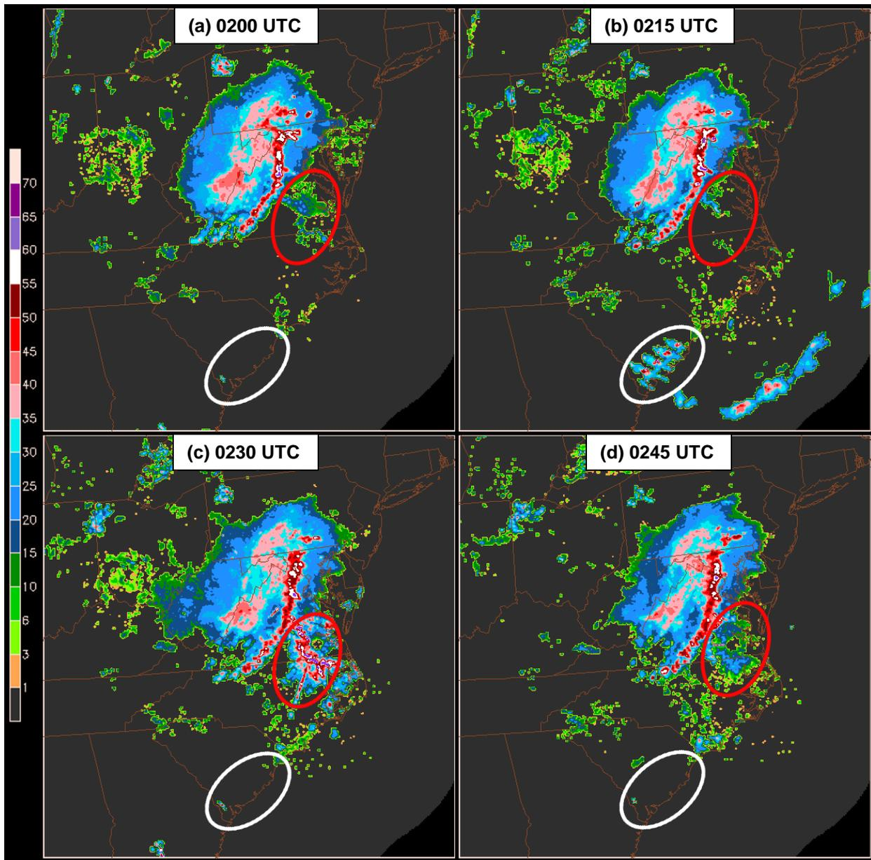
Figure 1. Example of temporally-transient false precipitation echoes in MRMS 5-km max CREF grids at 15-min intervals on 30 June 2012 (famous eastern US derecho). Anomalous propagation echoes just ahead of derecho (within the red ellipse) are quite weak at (a) 0200 UTC, almost non-existent at (b) 0215 UTC, very intense at (c) 0230 UTC, and moderate at (d) 0245 UTC. Microwave interference echoes within the white ellipse are present only at (b) 0215 UTC.
