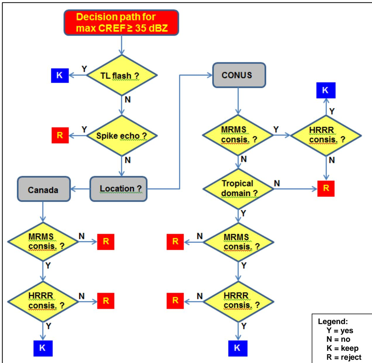
Figure 6. Dynamic QC decision tree, which is applied to maximum composite reflectivity (max CREF)  $\geq 35$  dBZ in a 5-km grid box. Diamond shapes with yellow fill denote individual tree decision modules, where “consis.” is an abbreviation for consistency. See Figure 7 and text for details pertaining to each decision module.
