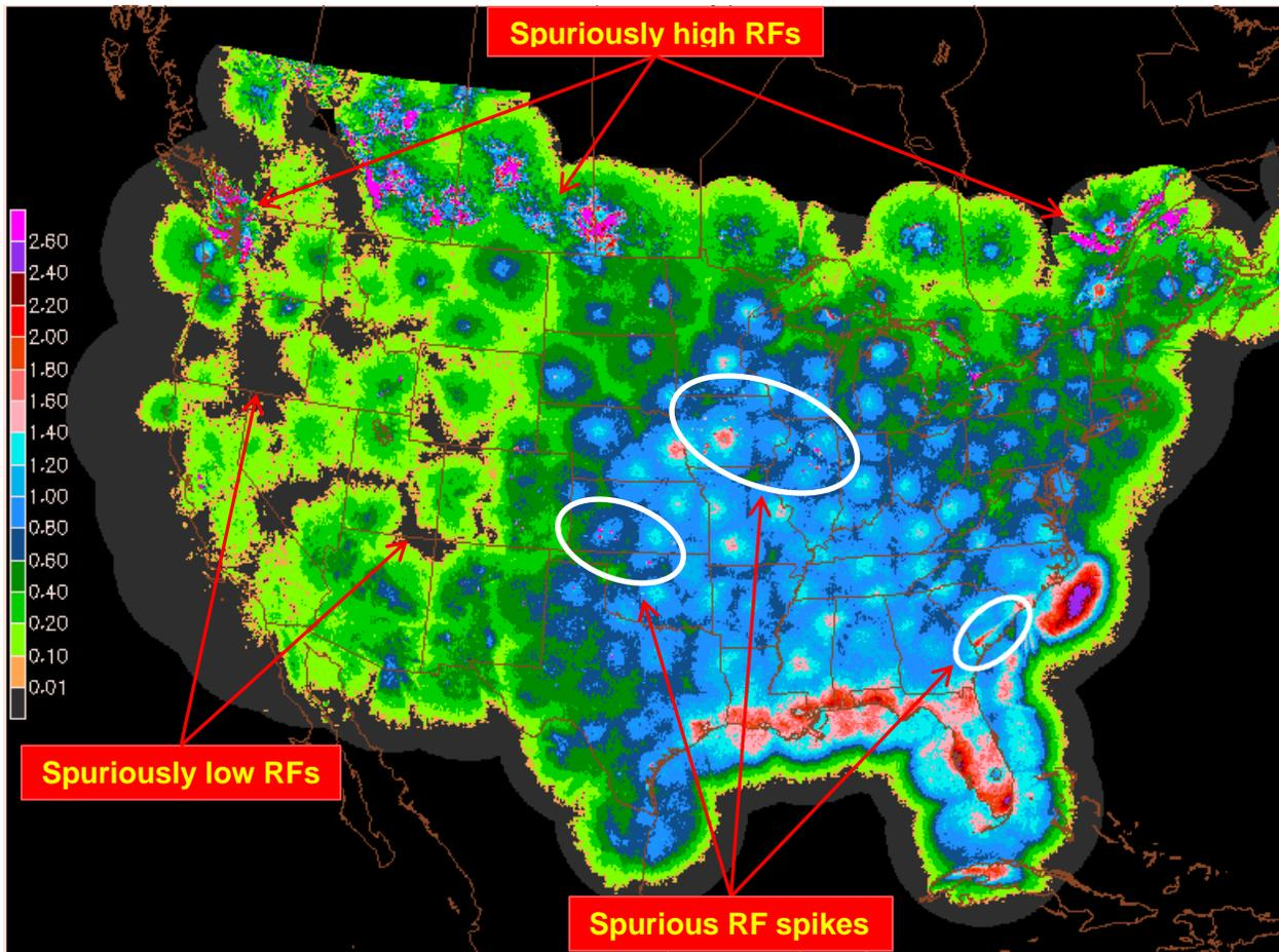
Figure 2. Relative frequency (RF; %) of max CREF  $\geq 40$  dBZ in 5-km grid boxes for the the warm season (April – September) of 2012-2016. Annotated RF features are discussed in the text.
