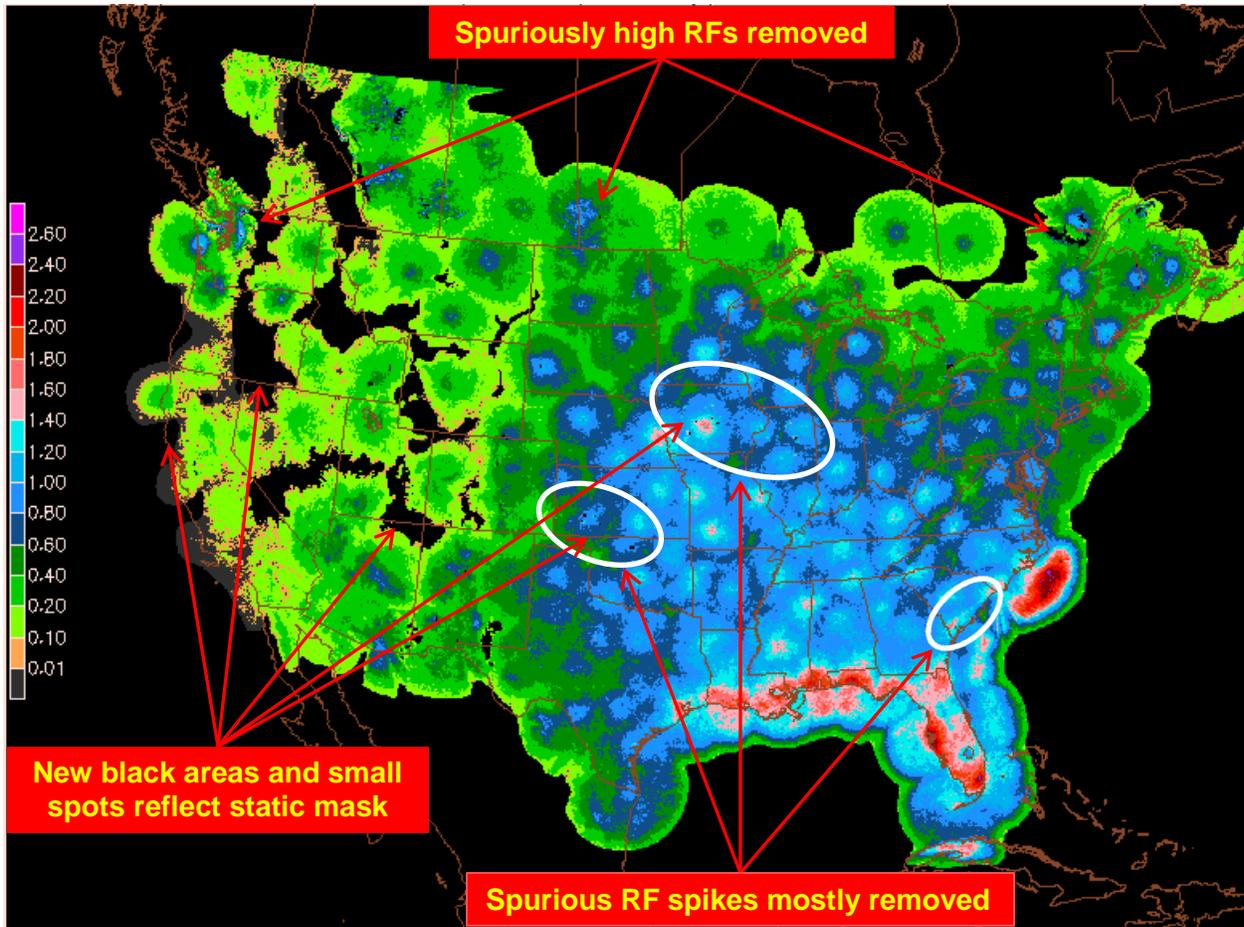
Figure. 10. Relative frequency (%) of CREF  $\geq$  40 dBZ for warm season after dynamic QC and static QC processes are applied to the base 5-km max CREF grids. Annotations are discussed in the text.
